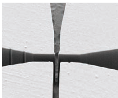
Figure 1. Detail of the channels of the new improved micromixer fabricated by DXRL.
